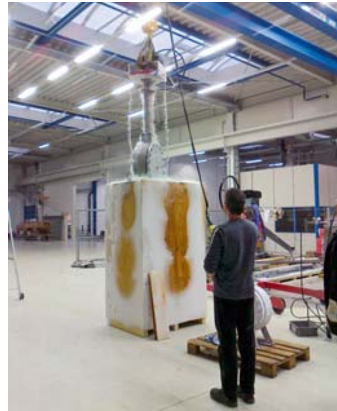
Even the biggest of the four offset butterfly valves was tested at maximum differential pressure at -196 °C with zero leakage
