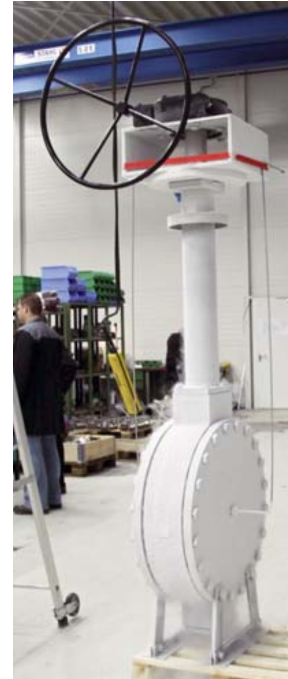
Even the biggest of the four offset butterfly valves was tested at maximum differential pressure at -196 °C with zero leakage
