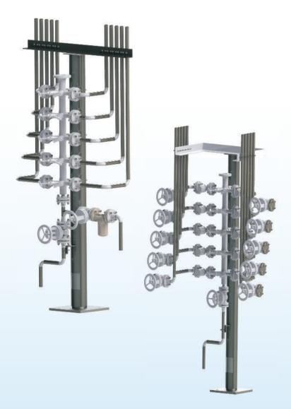
Compact elements of steam tracing (satellite) system, equipped with steam traps, manifolds with built-in shut-off valves, stop valves, piping, fittings and support elements. Their compact design saves space on the installation, and thanks to the workshop prefabrication method, construction, execution or corrosion protection is incomparably better, and the assembly itself becomes much faster and easier.
